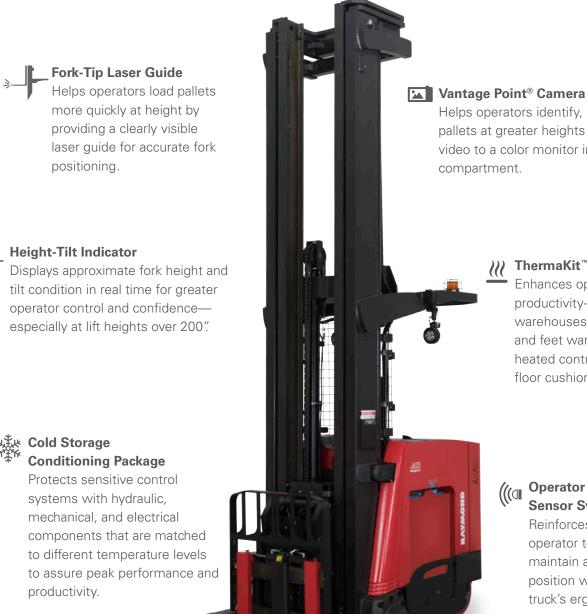
Helps operators identify, place and retrieve pallets at greater heights by relaying video to a color monitor in the operator compartment.
