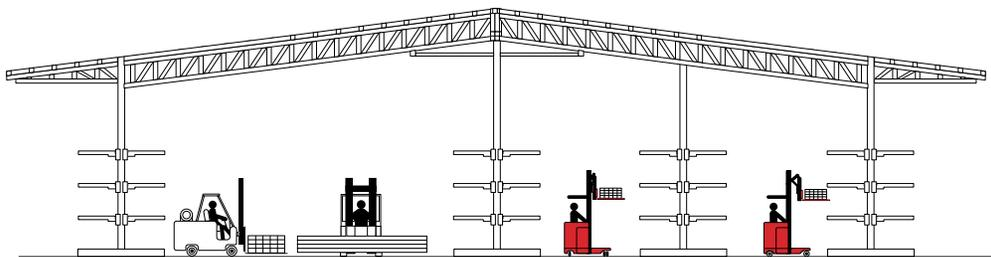
Conventional Storage: Using standard counterbalanced lift trucks, aisles must be wide enough to permit right angle maneuvering with long loads.
